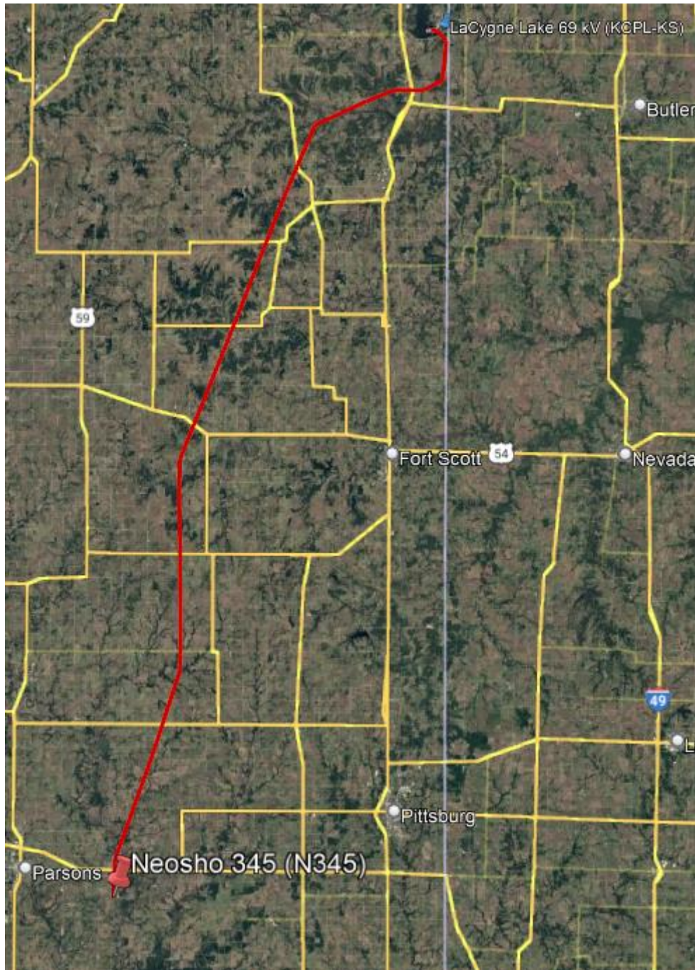
Figure 6 – LaCygne - Neosho 345kV Line
